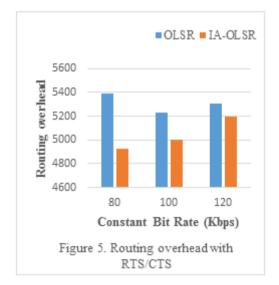
In the second simulation, the nodes move within the area of 550m x550m, Constant Bit Rate (CBR) changes from 80 Kbps to 120Kbps and turning off RTS/CTS.
